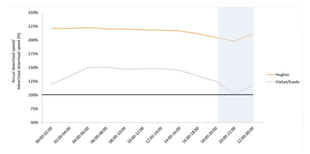
Chart 6 (in section 2.C) Illustrated, for each ISP, the ratio of actual download speed that was experienced by at least 80% of panelists for at least 80% of the peak usage period ("80/80 consistent download speed") to advertised download speed, and for reference the ratio of actual download speed to advertised download
